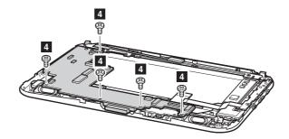
When installing: Make sure that all the connectors are attached firmly.
